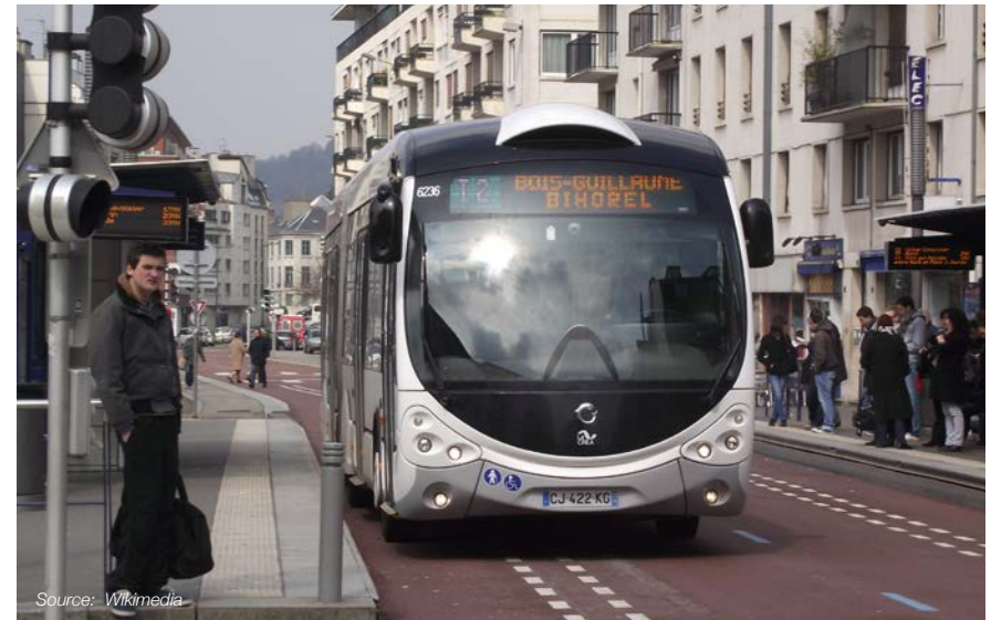
Figure 3-31: Irisbus low-emission diesel buses with wide doors and level boarding operated by Rouen
