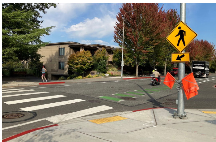
Existing marked pedestrian crossing with flags
