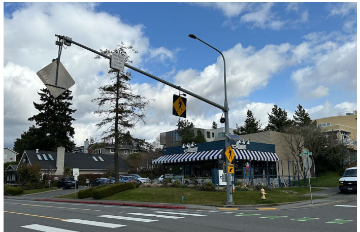
Overhead RRFB at NE 59th St
