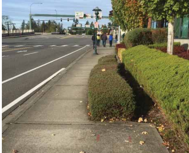
The clear walking zone should not meander or be interrupted by planting, such as this segment on NE 128th St.
