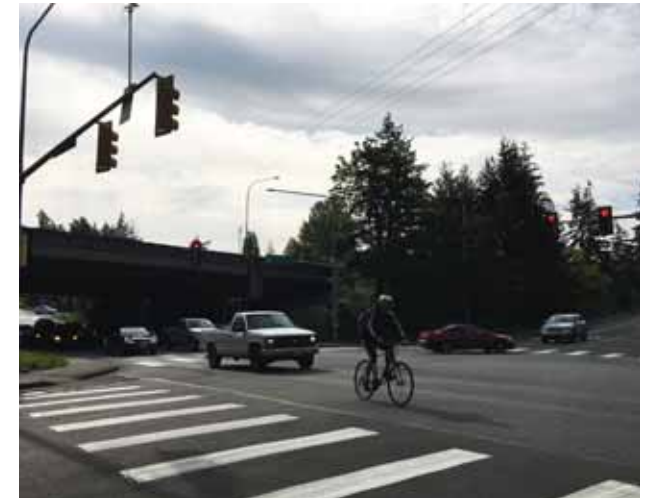
The intersection of NE 132nd St and 116th Way NE represents LTS 4 as there are no bicycle lanes, a wide street, and high vehicle speeds. This would be only comfortable for the most intrepid rider.
