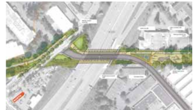
Street connection design concept beneath I-405 from the Cross Kirkland Corridor Master Plan. Note the proposed street would be a neighborhood connector street oriented to local traffic rather than arterial throughput.
