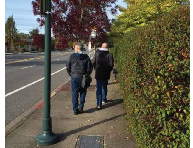
Utilities and plantings reduce the usable width for walking and a sidewalk. New developments should provide minimum buffer zone for utilities to be located outside of the clear zone.
