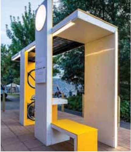
A bike hub is a small shelter with map information, tools, and a bicycle repair stand. These hubs can be integrated with transit shelters.
