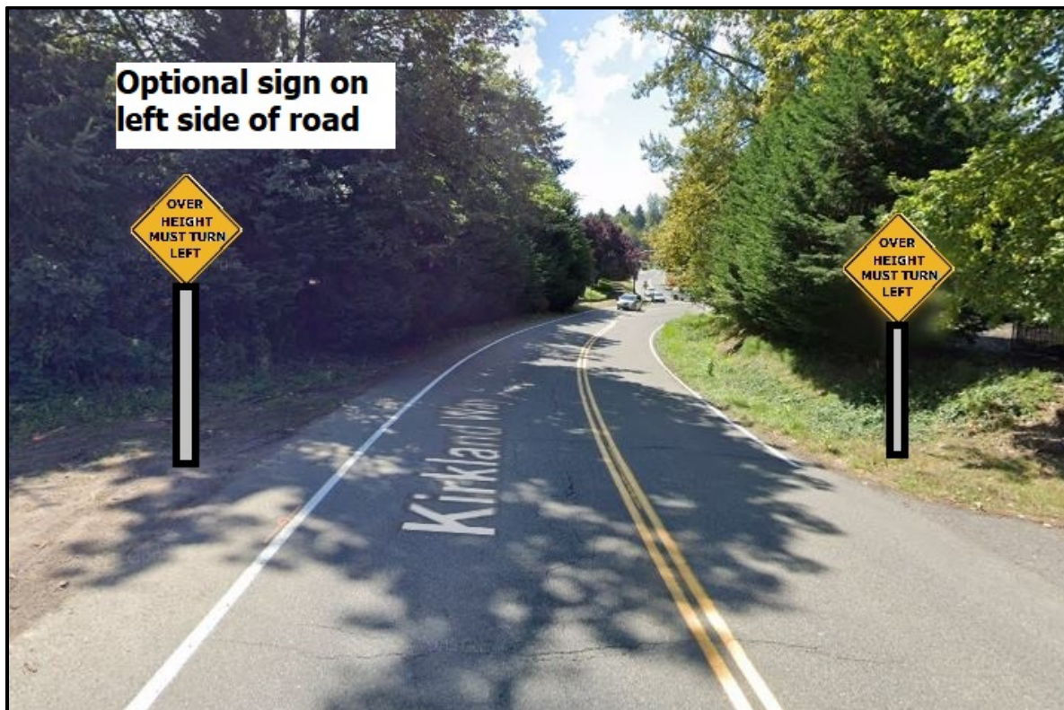
Figure 9 – Sign 4: “Over Height Must Turn Left” sign, optional sign on left side of road
