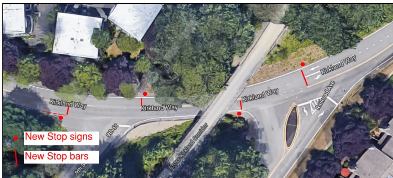
Figure 1. Option S-2a, Two Separate Three Leg All Way Stop Intersections
