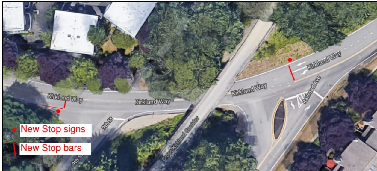
Figure 2. Option S-2b, Single Four Leg All Way Stop Intersection
