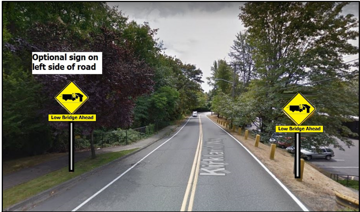
Figure 6 – Sign 1: Truck striking bridge with “Low Bridge Ahead,” optional sign on left side of road
