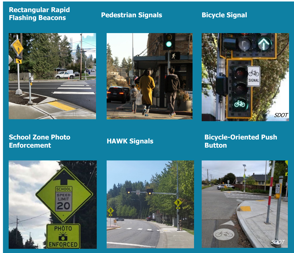
FIGURE 3-22 EXAMPLES OF TRAFFIC CONTROL DEVICES IN KIRKLAND
