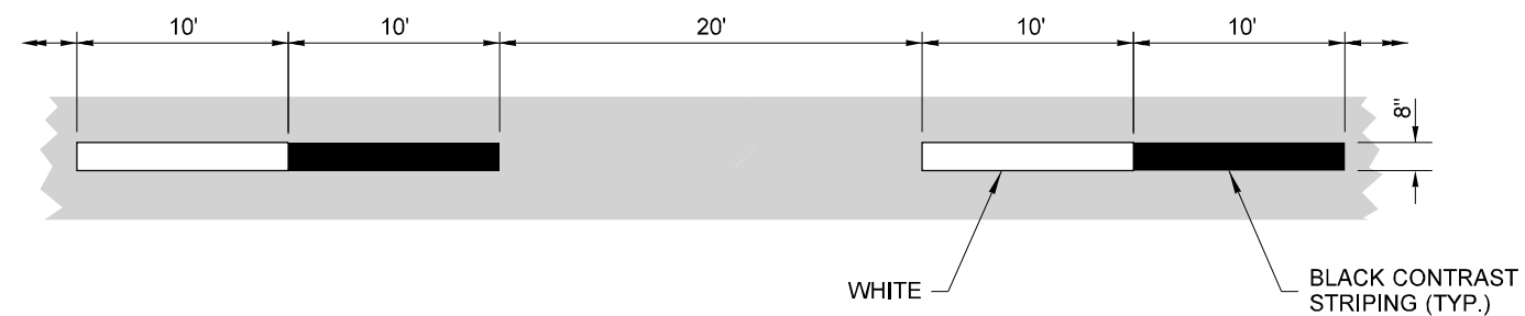
WIDE BROKEN LANE LINE
