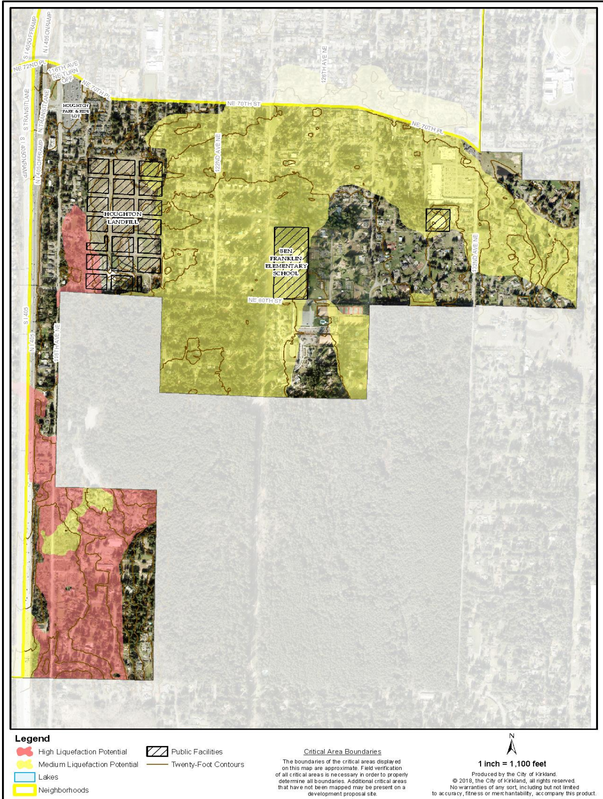
Figure BT-3: Bridle Trails Liquefaction Potential
