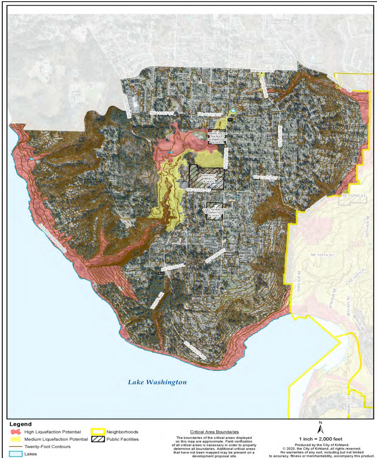
Figure FH-4.2b: Finn Hill Liquefaction Potential
