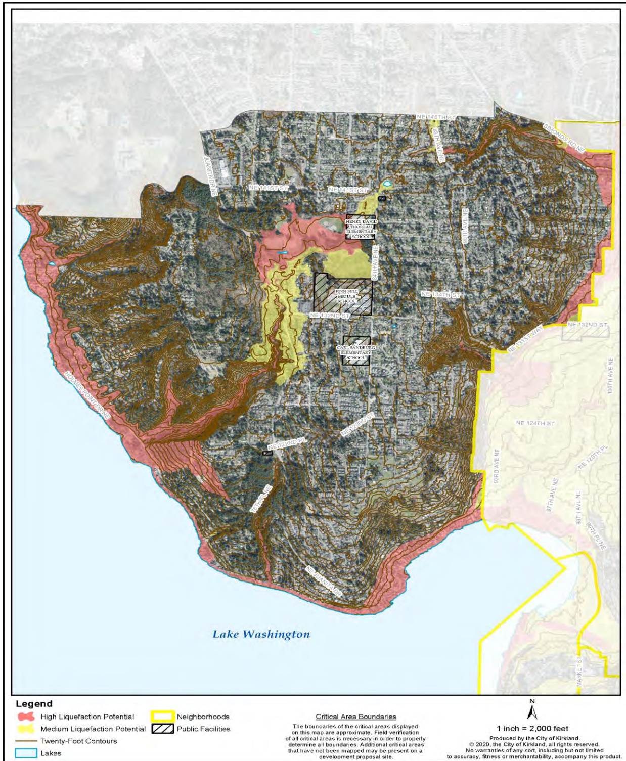
Figure FH-4.2b: Finn Hill Liquefaction Potential
