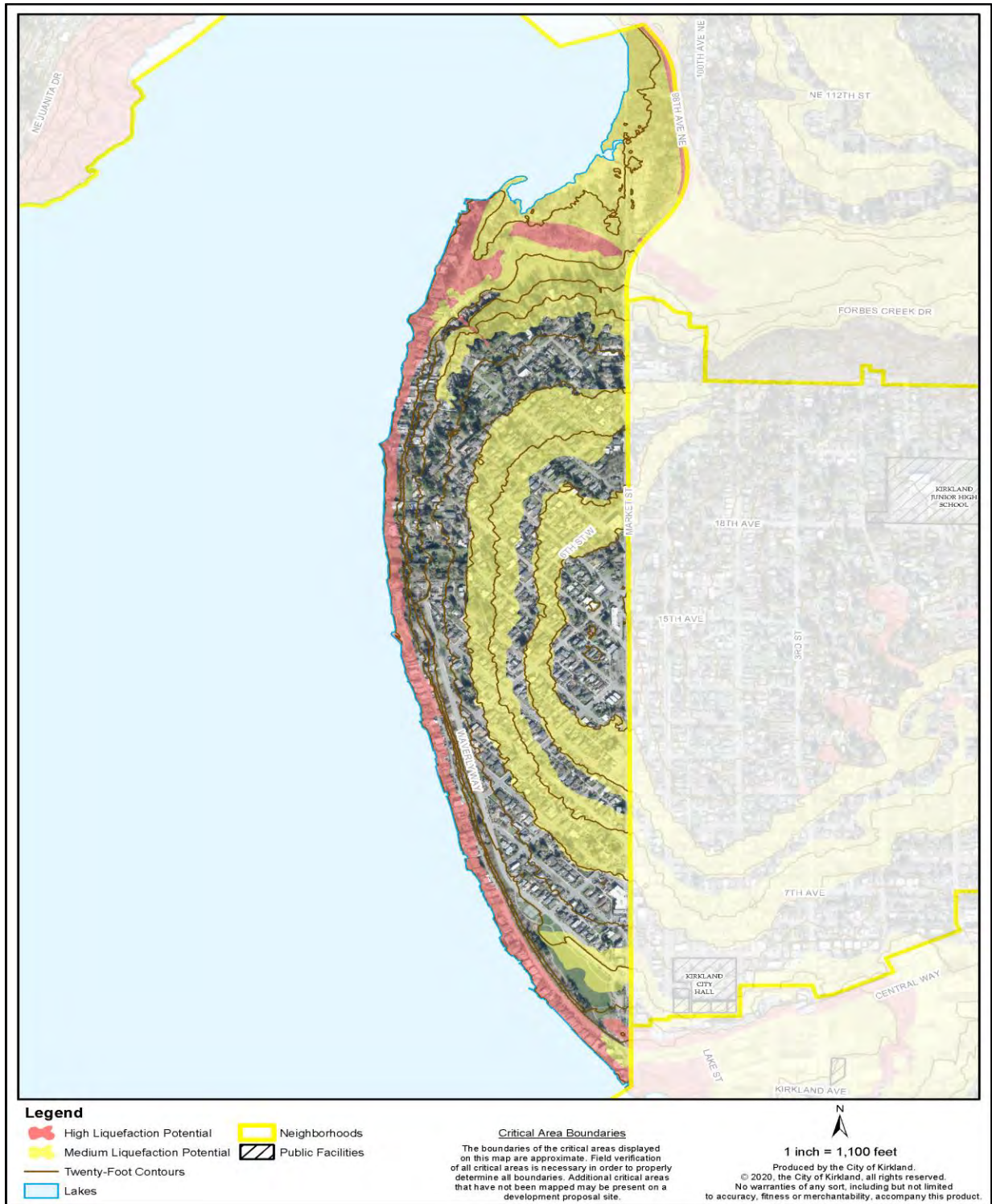
Figure M-2b: Market Liquefaction Potential
